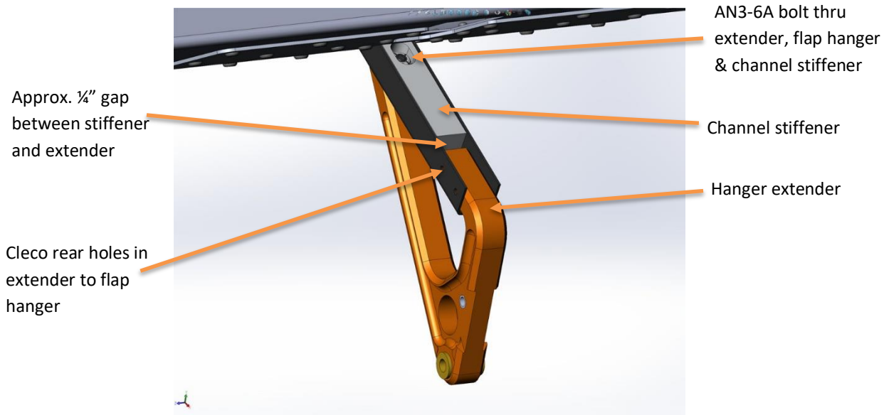
Figure 12: Extender and stiffener bolted to flap hanger
