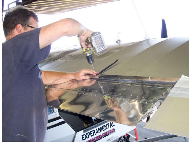
Figure 19: Install Gap Seals
