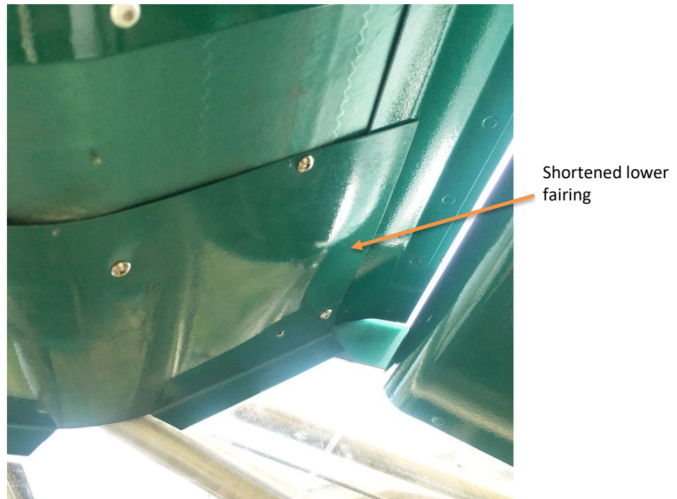
Figure 21: Lower wing root fairing modification
