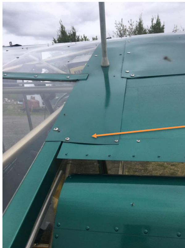
Figure 20: Upper wing root fairing modification
