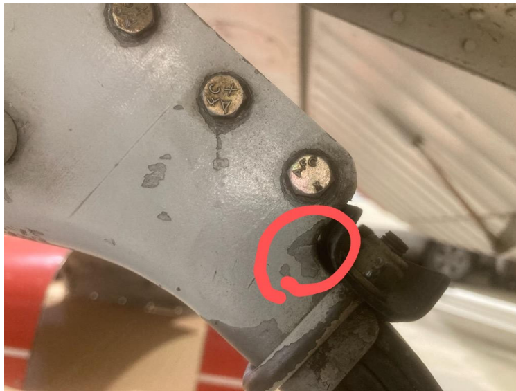
Figure 1: Crack Location in 0512154-1 Bracket (each side)
