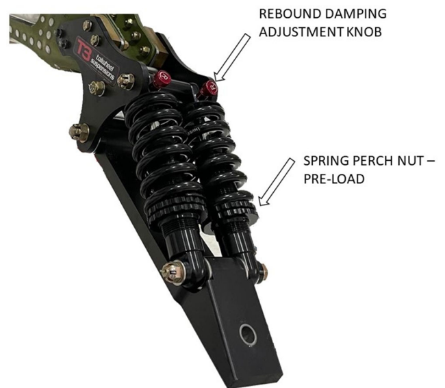
Figure 1: Shock Adjustment Locations
